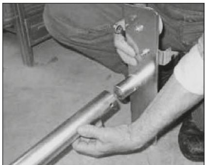
Mount slide guides with hexagon screw, flat washer and lock nut.
