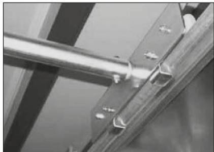
In use position, steps of shelf ladder must be as flat as possible. Set up ladder by adjusting the guide tube.
