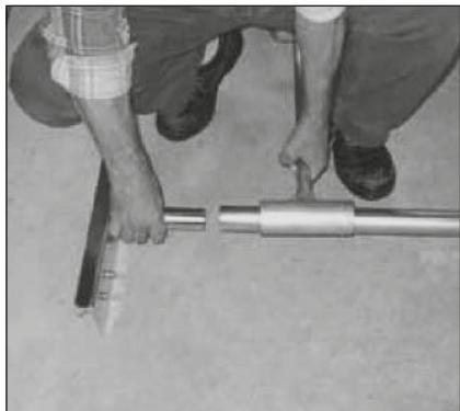
Slide head chassis over horizontal tube.
