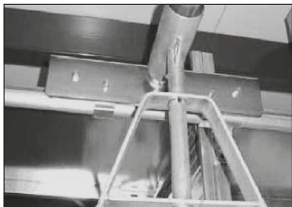
Please lift the ladder part. By turning 90 degrees, shelf ladder is kept in this position with cross pin.
